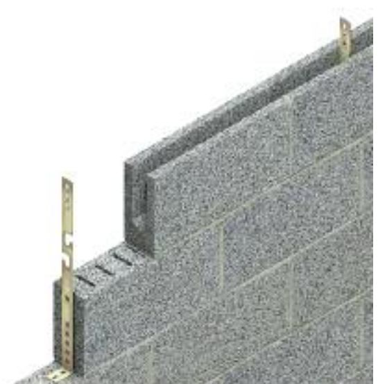
Step Two U-blocks installed as next course with transfer rods penetrating at midway point through slot at base of U-block. The slotted blocks below provide for an enhanced mortar bond, and rebated ends allow a standard vertical joint thickness to be maintained.
