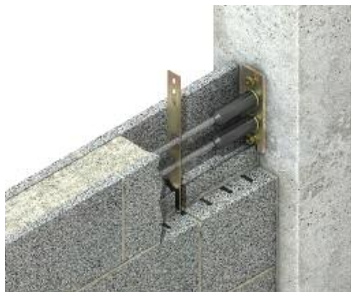
Step Four The reinforcement bars are inserted through the PVC sleeves, which allow for thermal movement, into the end cleat. Concrete is infilled along the length of the panel and tamped to level, with top blocks being layed within three hours.
