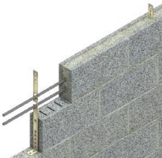
Step Three Reinforcing bar is passed through locating slots in the vertical transfer rod that ensures correct cover and bar centres. The bars should be lapped for 800mm between transfer rods when required.
