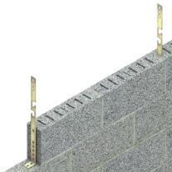
Step One The vertical transfer rods are fitted at perpend between slotted blocks at 900mm centres and mortared in place. The end cleats are fixed at either end of panel to concrete or steel columns.
